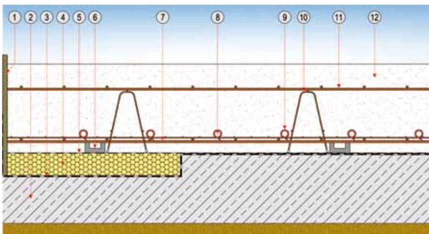
**System design industrial space heating with cable ties / with edge insulation**
