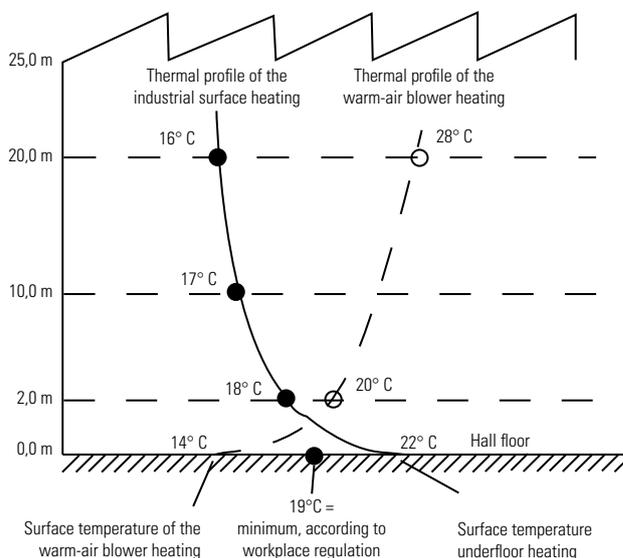
The commercial and industrial surface heating meets the requirements of the Workplace/- Directive without the partly required support measures (e.g. floor grates against cold feet) of other types of heating in an advantageous manner.
