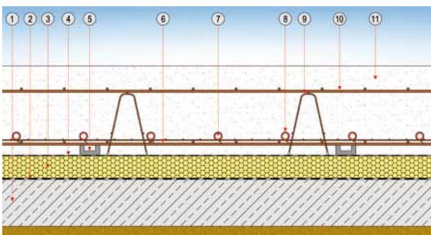
**System design industrial space heating with cable ties**
