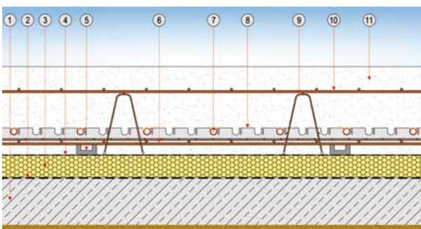
**System design industrial space heating with spring rail**
